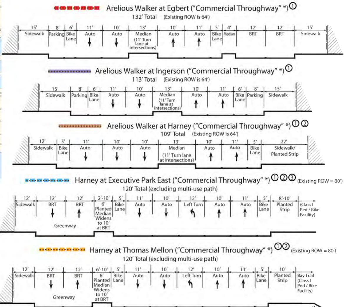
Sidewalks shall increase to 15' at bus rapid transit stops and shall conform to Better Streets Plan guidelines for all other stops (typical)
