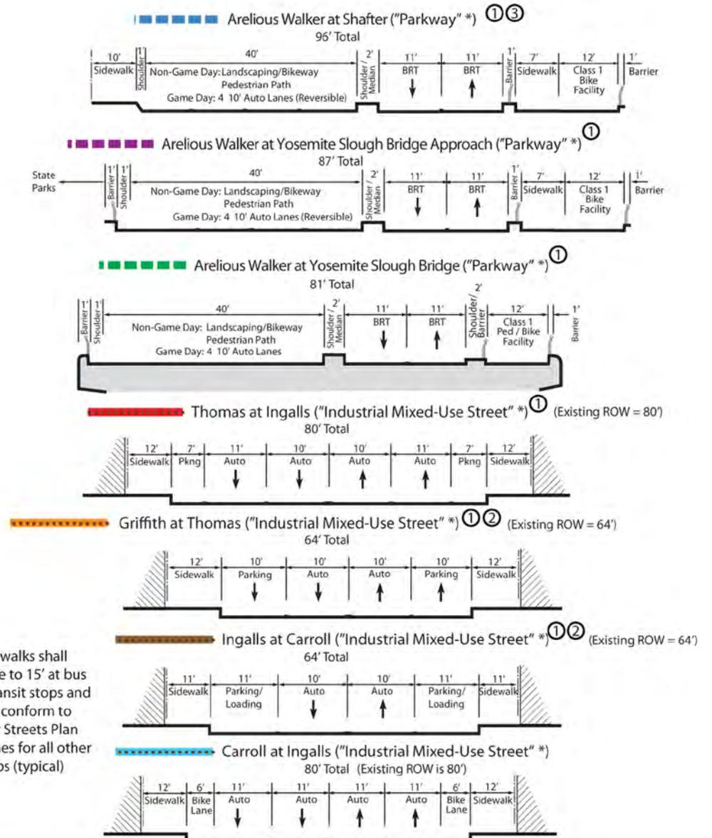
Sidewalks shall increase to 15' at bus rapid transit stops and shall conform to Better Streets Plan guidelines for all other stops (typical)
