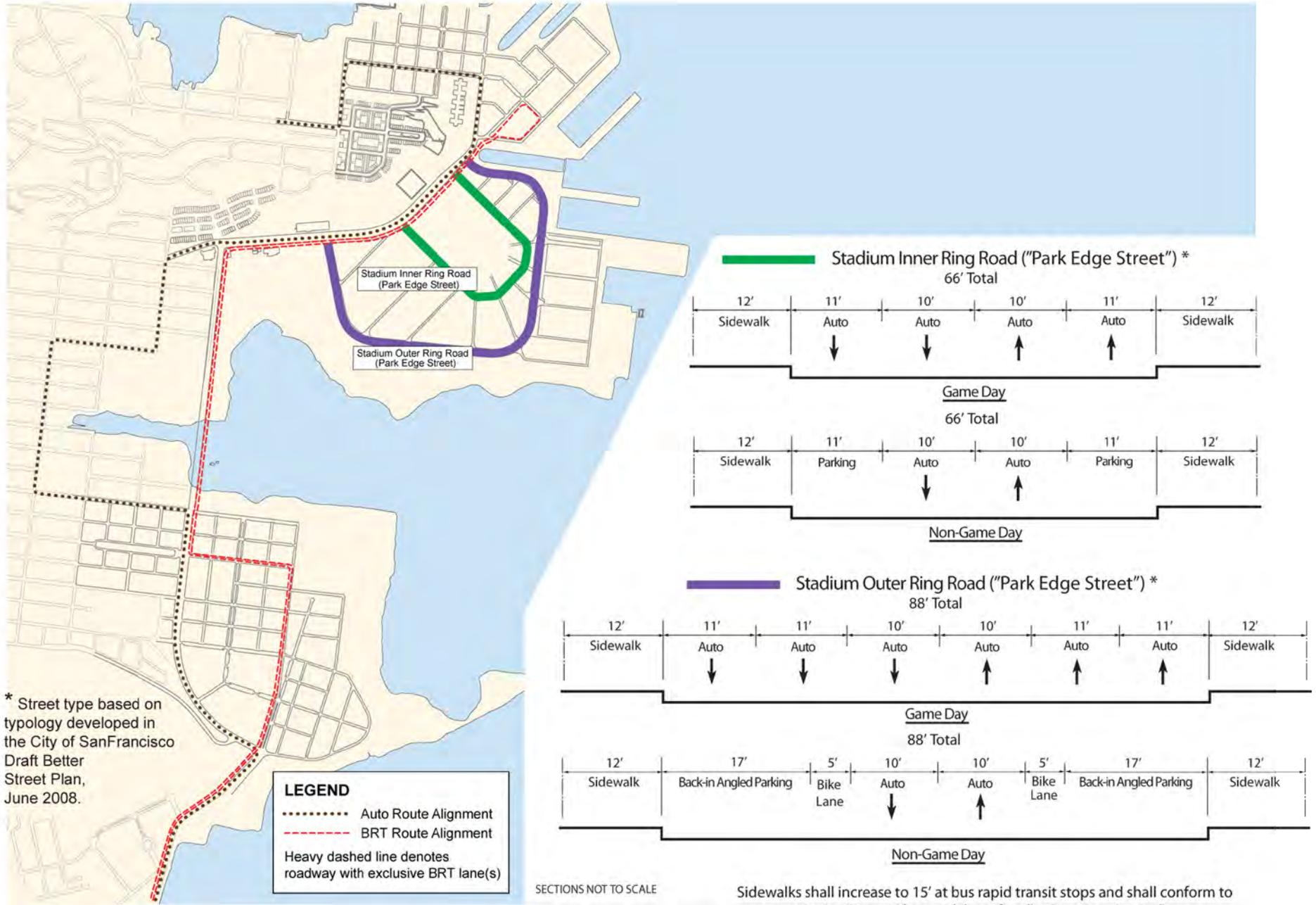
Sidewalks shall increase to 15' at bus rapid transit stops and shall conform to Better Streets Plan guidelines for all other stops (typical)
