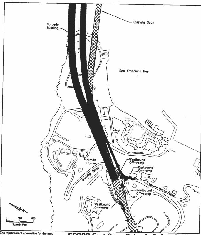
The replacement alternative for the new east span of the SFOBB is north of the existing span. Existing Yerba Buena Island on- and off-ramps are also shown. The redesign of new ramps on Yerba Buena Island is the subject of continuing discussion between Caltrans and the City and County of San Francisco.
