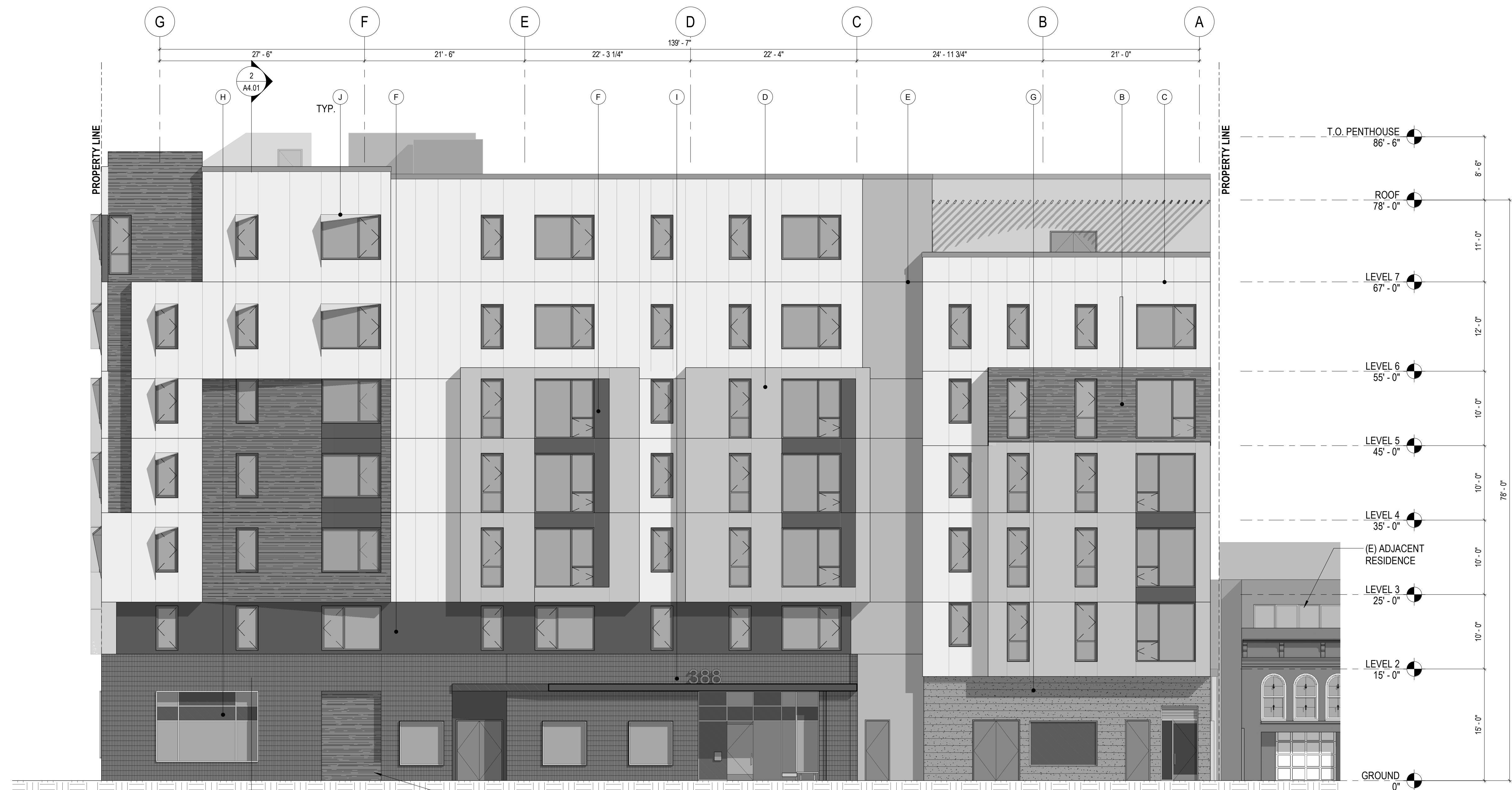
1 PROPOSED - EAST ELEVATION 1/8" = 1'-0"
