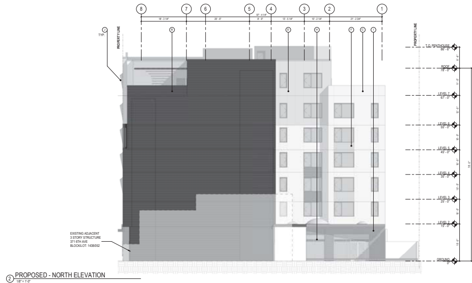
① PROPOSED - NORTH ELEVATION 1/8" = 1'-0"
