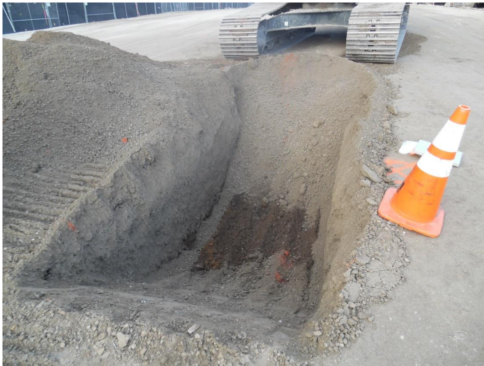
Photograph 8: 5/22/15 – Bottom of test pit from Photograph 6 showing the color and grade change between the crushed concrete cap material and the earthquake fill.
