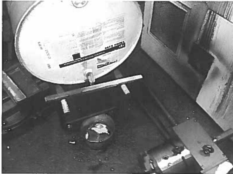
Photo 1. View of inverted 55-gallon drum of cutting oil with dispenser; floor is wet from apparent leaks and spills (Photo date: March 29, 2013).
