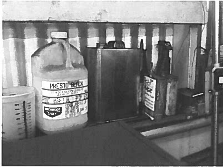
Photo 1. View inside Production Specialties of cutting fluids stored on shelf, including several listed as containing chlorinated hydrocarbons (e.g., trichloroethylene) (Photo date: March 29, 2013).
